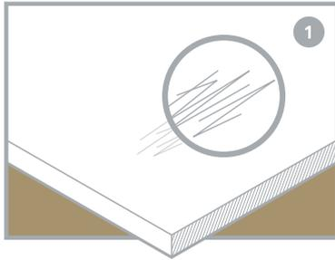
Superficial defects caused by micro-scratches.
