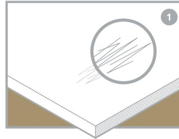
Superficial defects caused by micro-scratches.
